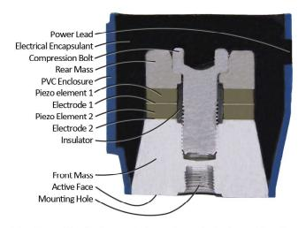
The CleanAHull ultrasonic transducer is designed for the harsh marine environments effective on a wide range of hulls including Steel, Aluminium, GRP (Fibre Glass), Carbon Fibre, Kevlar, HDPE and more.
